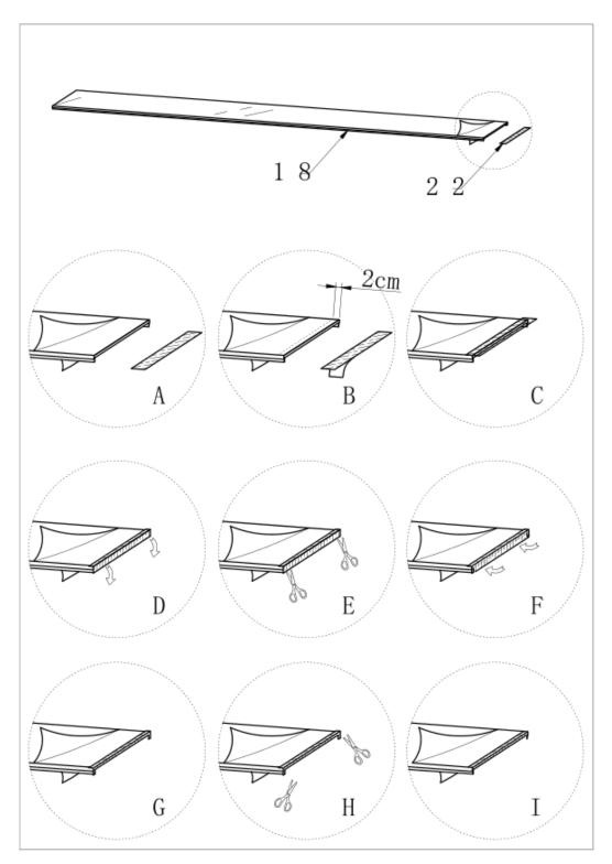
Begin installing the first polycarbonate panel (18) as shown below. Make sure the panel is touching the wall mount rail (1) as shown in figure (i). (The side sealed with <u>part 22</u> should be on the lower side)
