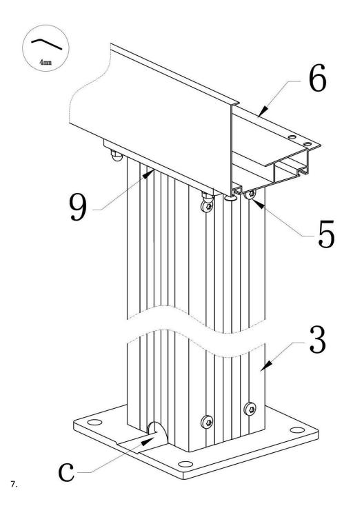
Using the side rail (11) attach the front rail and supports (3) to the wall mount (1). Make sure the threaded holes on the side rail (11) are on the outside (e), then attach using M6 x 16 hex screws (5). **Do not install the second side rail until you have completed the next step!**
