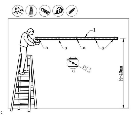
Using a 12mm  $\emptyset$  drill bit, drill holes 80mm deep at each point marked (a). This will allow installation of the expansion bolts (2). If the product is being mounted to a wood surface, substitute expansion bolts for coach bolts or coach screws. This will depend on the exact application and is at the customer's discretion.
